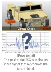
Iterative search algorithm used to generate the drive signal to reproduce the target signal in the virtual model
