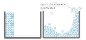
Particle-based CFD methods easily handle free surfaces and moving boundary geometry, and no mesh is used.
